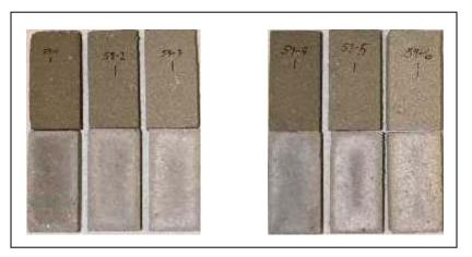
Figure 4 - Paver mixes with 13.6% (left set) and 18.3% (right set) cement Water-cement ratios are 0.28, 0.35 and 0.42 from left to right in each set Top row show surfaces that were open to the air during drying Bottom row show surfaces that were against the lab bench during drying
