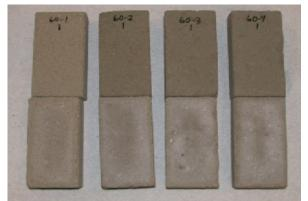
Figure 2 - Increasing cement contents (left to right)
